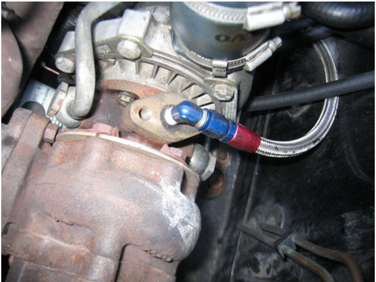
Garrett T3 oil feed flange with 4AN outlet.
